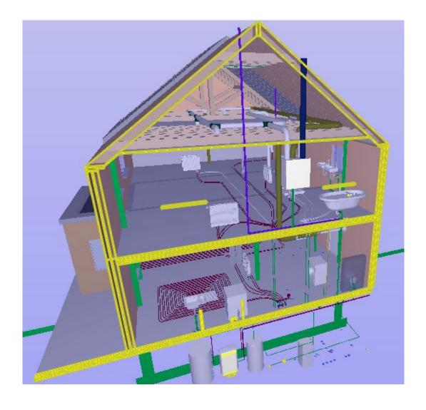
Discover the different techniques (one at a time) (heating, sanitary, drainage, electricity, ventilation) and then see them together to highlight the need for collaboration between the trades
